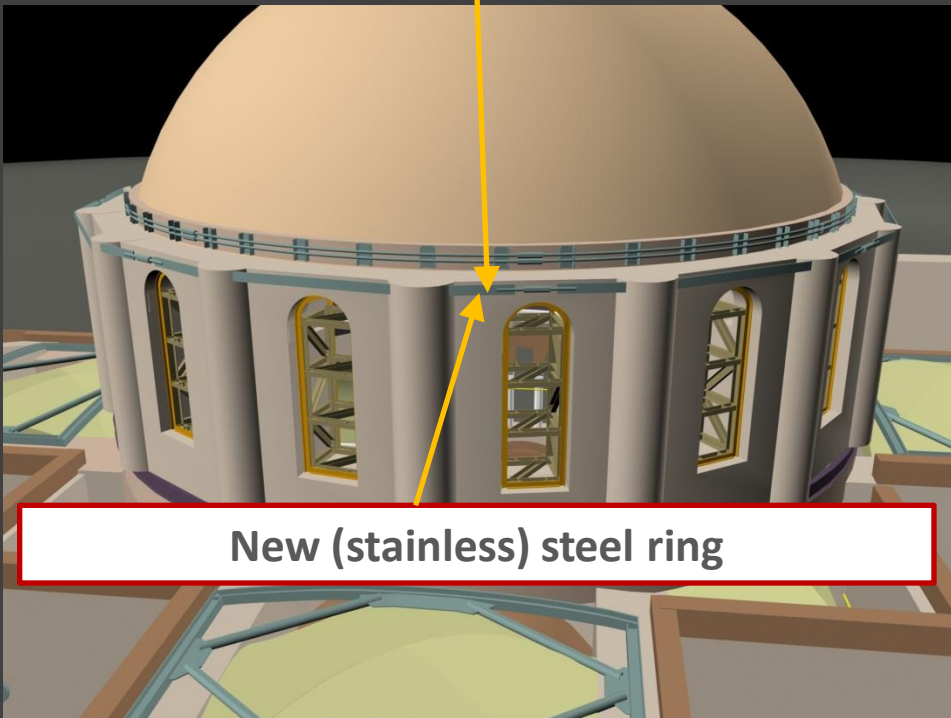
New (non visible) steel ring at the extrados of the cupola
