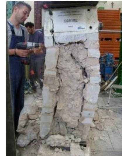
Increase of approximately 2 times of the compressive strength for both scales (slightly higher for the 2:3 scale specimens).
