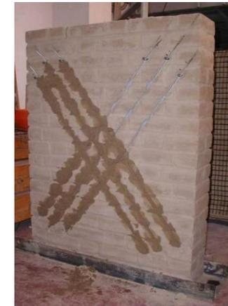
Adobe brick wall with a steel wire ropes (ABW\_2)
