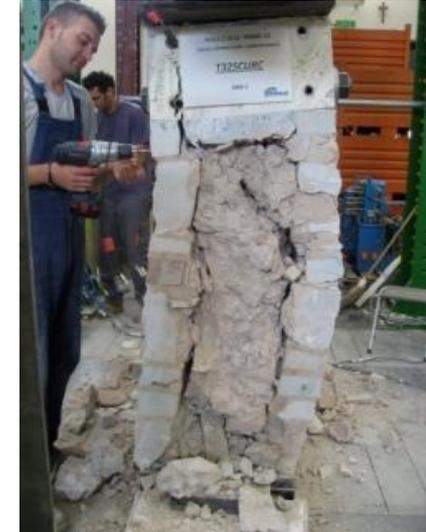
Increase of approximately 2 times of the compressive strength for both scales (slightly higher for the 2:3 scale specimens.
