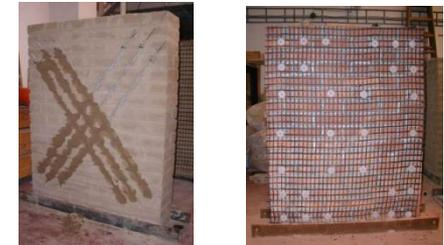
GEOGRID AND STEEL WIRES FOR BRICK AND ADOBE WALLS (ITAM)
