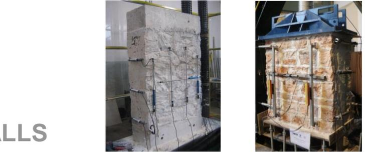
GROUT INJECTION OF EARTHEN WALLS (BAM)
