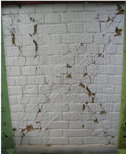
Reinforced samples with steel wire ropes (ABW\_2)
