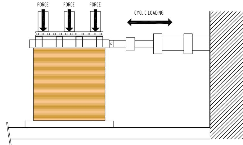
Compressive loading: 140 kN. The vertical compressive prestress was combined with cyclic horizontal loading mode with a stepwise increase in the maximum cycling limits.
