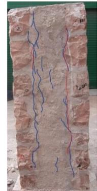
Failure mode in compression before (red line) and after (blue line) grouting of a) W. 2 and b) W. 4
