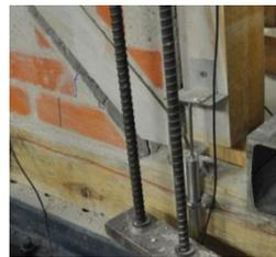
Unreinforced walls characterized by flexural behaviour, with posts uplifting → strengthening of connections to **prevent uplifting** and **improve shear behaviour**
