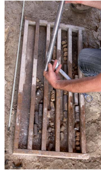
Figure 77. Extraction of Core Sample. Overview.
