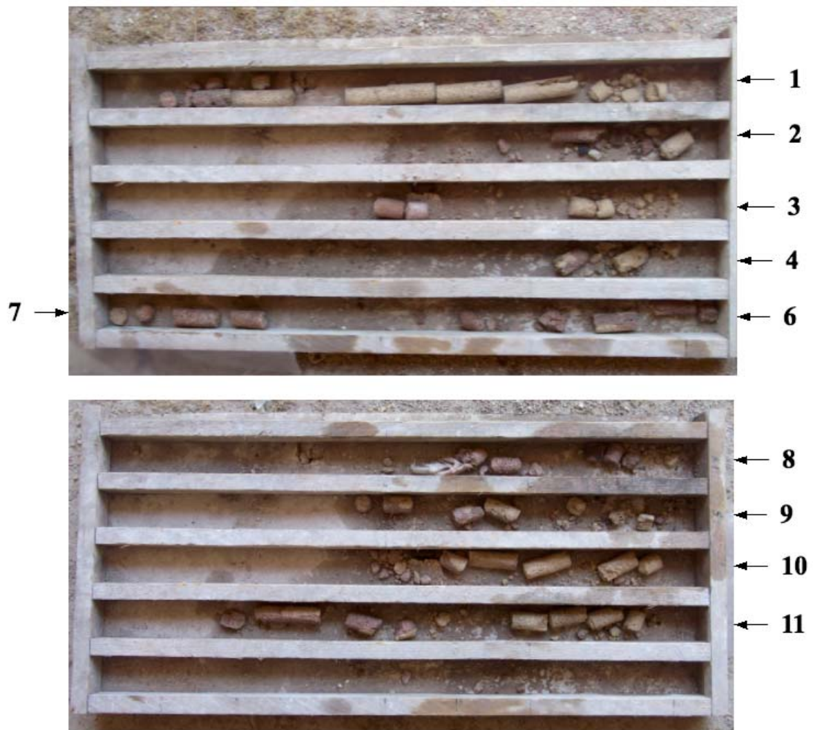
Figure 89. Core Samples, Vault 1 (No Material Extracted During Drill #5).
