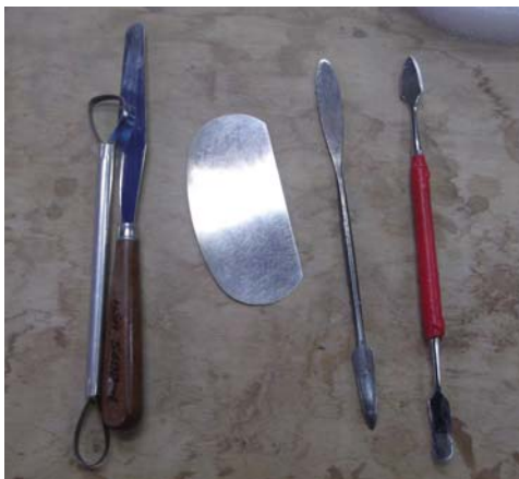
Above: Img. 39 Tools used for mixing, filling, and working plaster, Kowalchuk 2014
